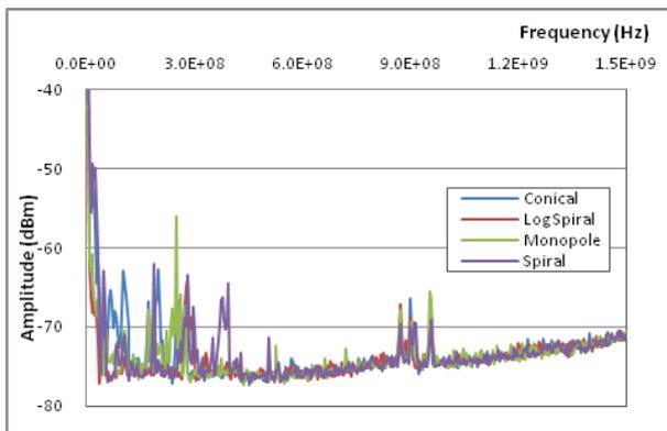
Figure 4. Full-span of void PD spectrum captured by 4 different sensors at 60 pC.
