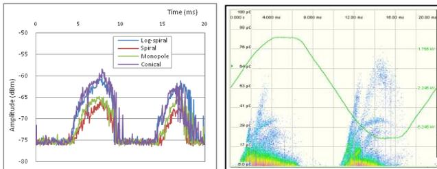
Figure 10. Zero-span spectrum at 270 MHz of the floating metal and comparison to the IEC60270
