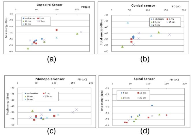
Figure 12. Total energy of zero-span with varying barrier position, floating metal PD source
