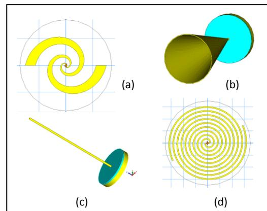
Figure 2. The types of sensor in use, (a) Log-spiral, (b) conical, (c) monopole, and (d) spiral
