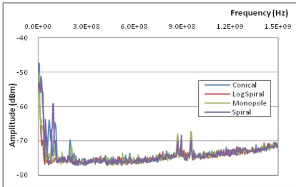
Figure 3. The background noise spectrum recorded by 4 different sensors.
