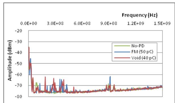
Figure 9. The full-span spectrum of floating metal and void, measured using spiral sensor.
