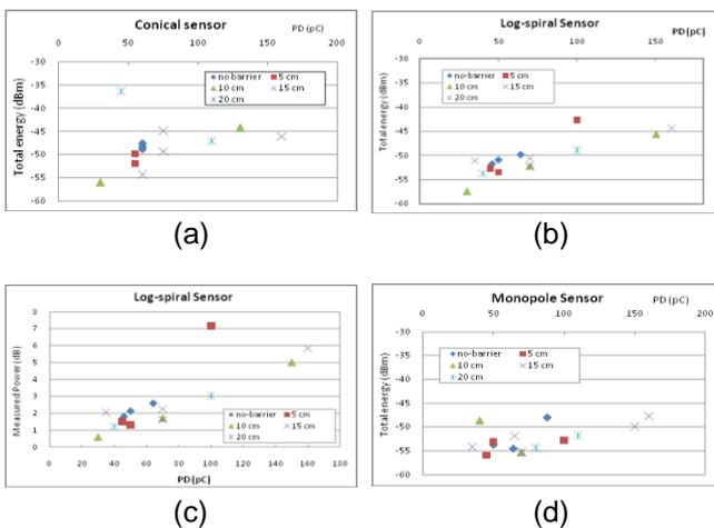
Figure 11. Full-span total energy of sensors with varying barrier position, floating metal PD source
