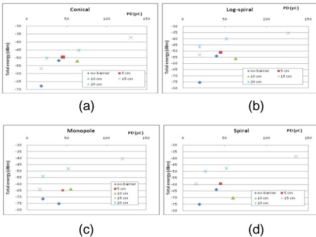
Figure 7. Total energy of zero-span spectra with varying barrier position, void PD source
