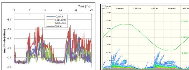
Figure 5. PD spectrum of zero-span at 270 MHz of void PD at 60 pC
