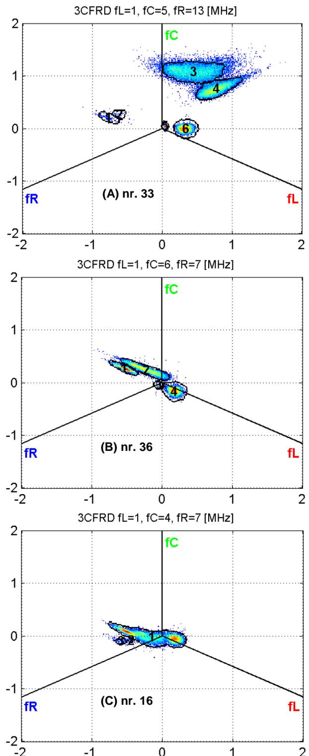
**Figure 9:** Clustered 3CFRDs for (A) frequency triple 33, (B) frequency triple 36 and (C) frequency triple 16 (see Figure 8)
