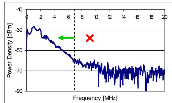
**Figure 5:** FFT of PDs of machine stator at 7.7kV test voltage
