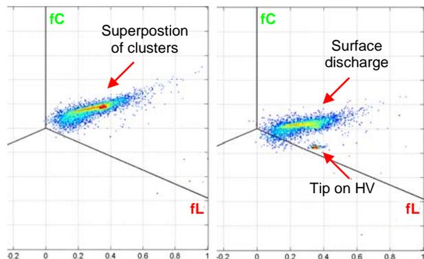
**Figure 3:** 3CFRDs for center frequencies 0.5, 3, 10 MHz (left) and 0.5, 4, 10 MHz (right), BW 650kHz
