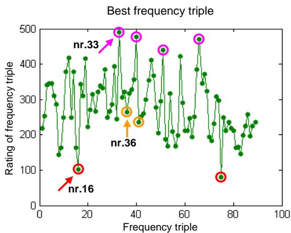
**Figure 8:** Rating of 89 different frequency triples for test setup with four artificial PD defects
