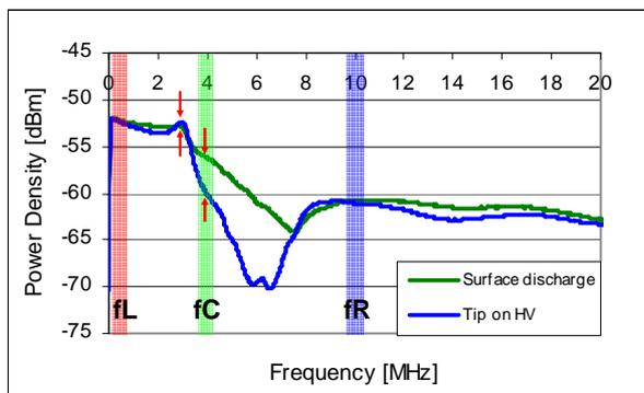
**Figure 1:** FFT of surface discharge and tip on HV in a test setup
