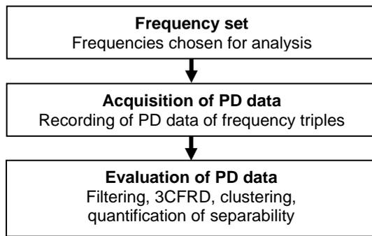
**Figure 4:** Block diagram modular software for automated determination of frequencies for 3CFRD
