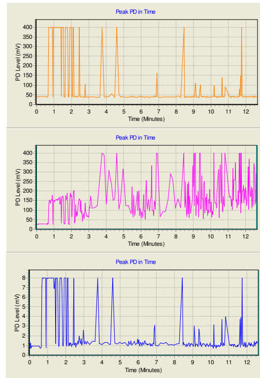
Figure 10, PD Activity vs Time during DC Ramp Up in Voltage, Chan 1 TEV down fibre (Gain 3), Chan 2 CT down fibre (Gain 3 means full scale =12600pC), Chan 3 Aerial measured directly
