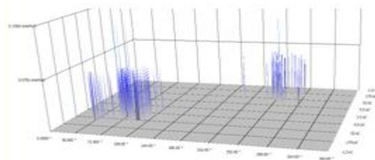
Figure 3: 3-D histogram of PD of clean paper-oil insulation
