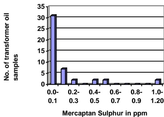
Figure 7: Measured mercaptan sulphur values in a sample survey of 50 power transformers
