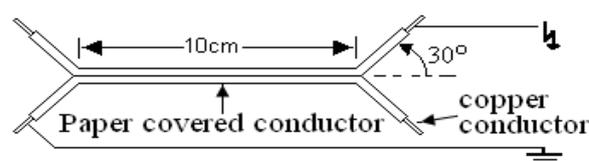
Figure 1: Specimen configuration for laboratory ageing studies
