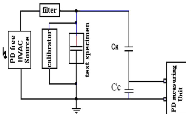
Figure 2: Partial discharge measuring circuit
