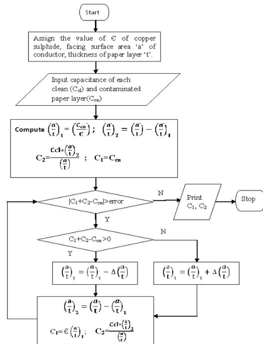
Figure.6: Flow chart for the evaluation of components of capacitive model
