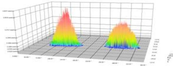
Figure 5 3-D histogram of PD of clean pigtail sample in contaminated transformer oil of failed power transformer
