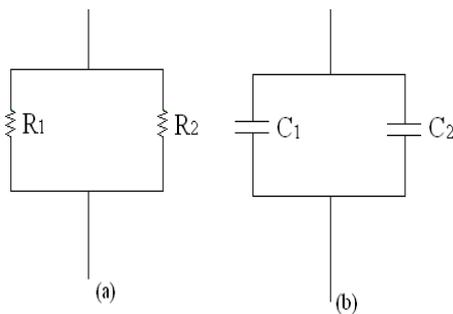
Fig.5 Equivalent circuit representation of copper sulphide partly contaminated single layer paper –oil insulation in
