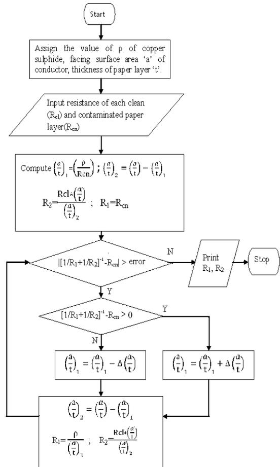
Figure 5: Flow chart for the evaluation of components of resistive model
