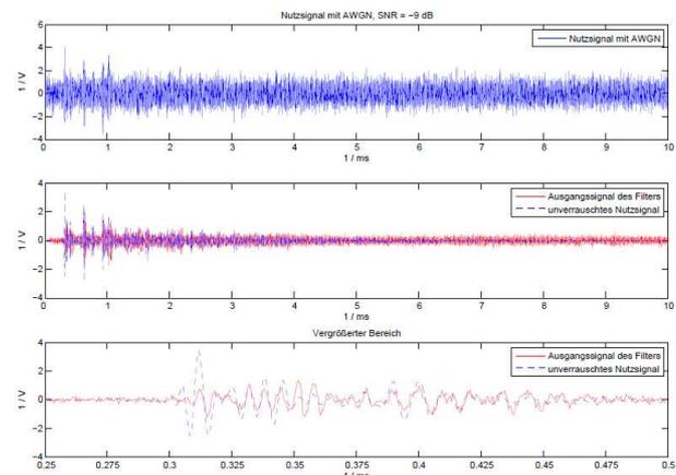
Figure 7: LMS filter signals
