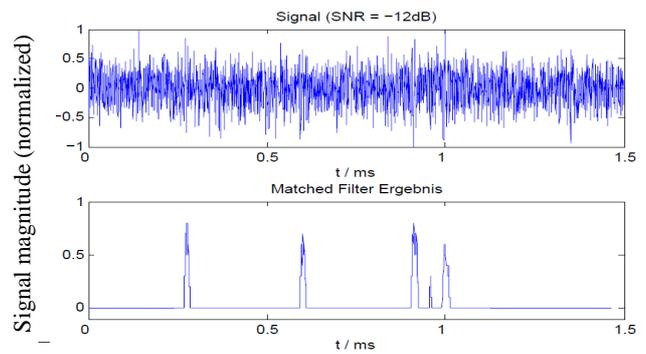
**Figure 11:** Matched filter result ( $SNR = -12dB$ )
