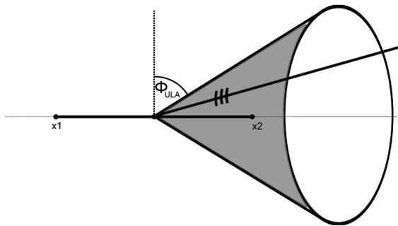
Figure 3: Ambiguity cone of one sensor pair
