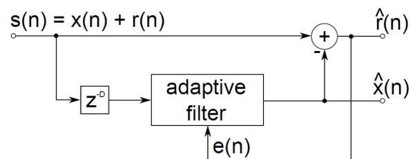
Figure 6: LMS filter structure
