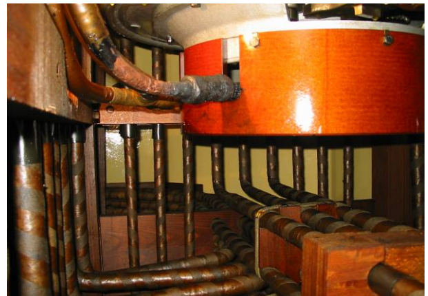
Figure 4: paper carbonisation and burning out phenomena on the OLTC connection
