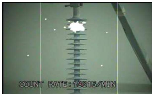
Figure 13: Result of the laboratory test with UV camera for aged insulator with pollution level 1
