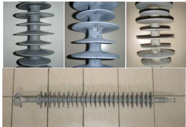
Figure 1: Polymeric insulators, class 72.5 kV
