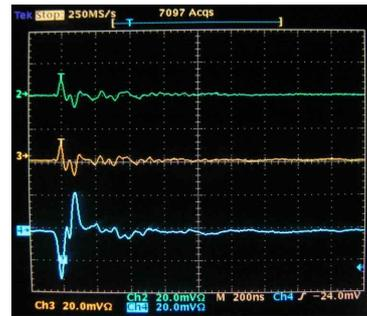
**Figure 3:** Characteristics of simulated pulse injected at 10m cable position
