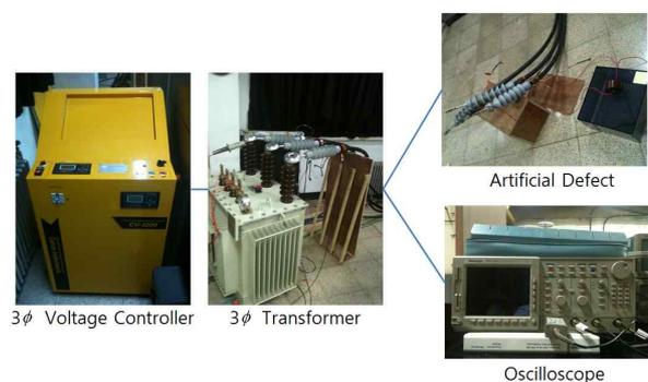
**Figure 1:** 3 phase PD experimental system
