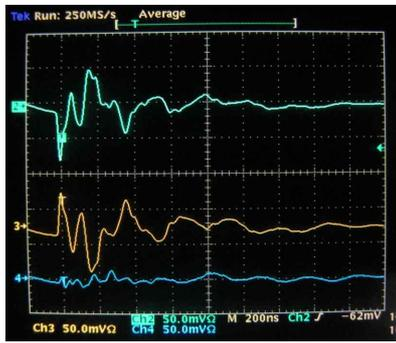
**Figure 7:** Characteristics of simulated pulse injected between two terminals of the transformer
