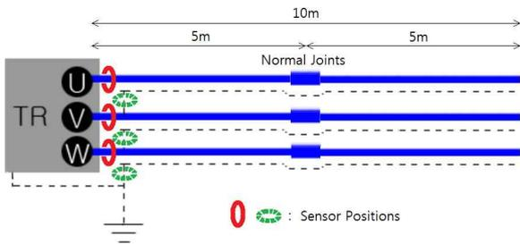
**Figure 2:** The layout of the 3 phase PD experiment
