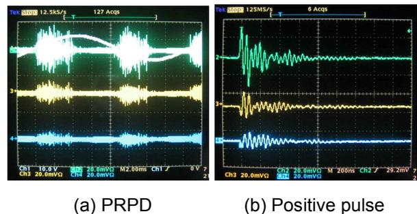
**Figure 4:** Void discharges from U-phase(CH2) 10m cable position
