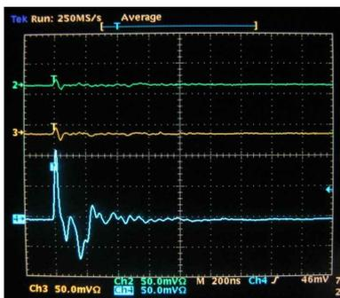
**Figure 5:** Characteristics of simulated pulse injected at 0m cable position
