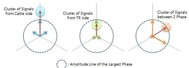
**Figure 9:** The new concept of 3PPAD considering pulse polarity and amplitude
