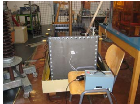
Figure 5. Position of Sensor 3 attached on the Tank
