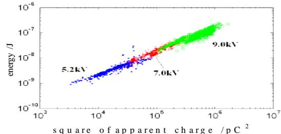
**Figure.9** Relationship between UHF signal and charge quantity at different voltage
