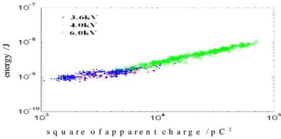
**Figure.7** Relationship between UHF signal and charge quantity at different voltage
