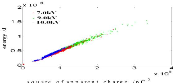
Figure.5 Relationship between UHF signal and charge quantity at different voltage
