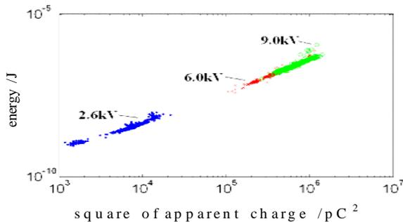
**Figure.11** Relationship between UHF signal and charge quantity at different voltage
