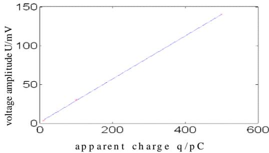
Figure.3 Calibration curve of pulse current method
