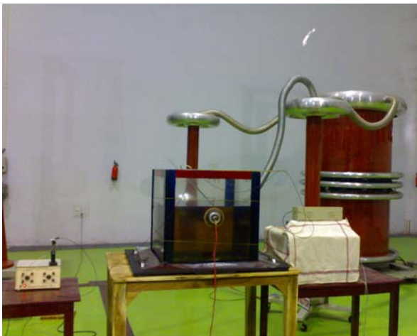
Fig. 2. Direct optical detection of PDs measurement setup.
