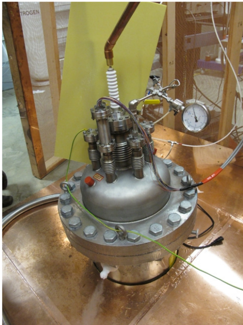
Figure 5: Photograph of the pressure cryostat, partially lowered into the laboratory floor; the G10 plate behind the bushing is for illustrative purposes only.
