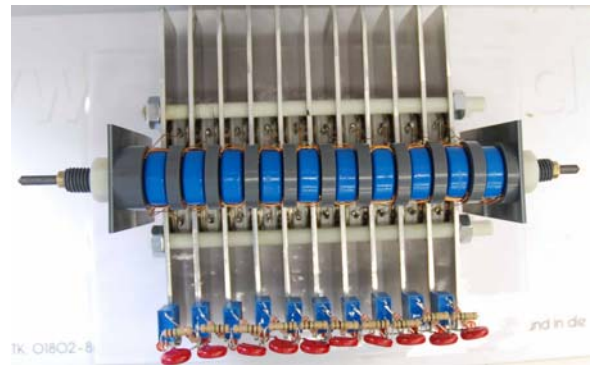
Fig. 7: Insulated impulse transformers of the ac switch, mounted on one common primary conductor
