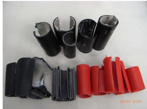
Figure 7: Cable sheath probes prepared for the indirect determination of breakdown voltage U_d
