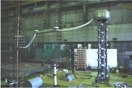
Figure 8, Setup of DC voltage breakdown test
