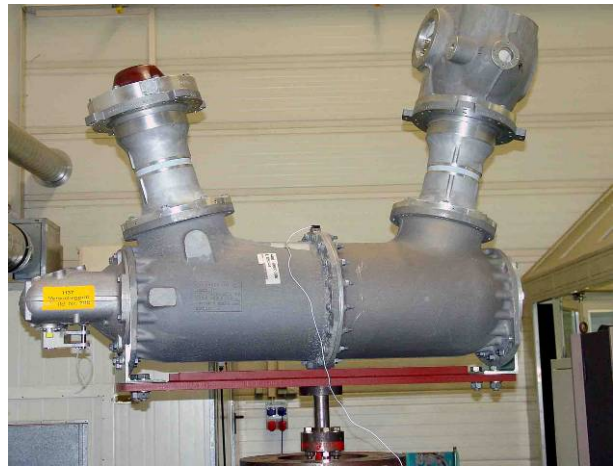
Figure 7: Example of a transportation test of a 145 kV DT-Breaker
