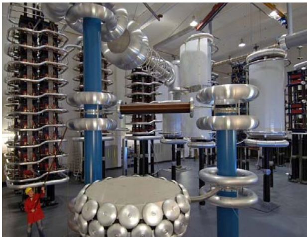
Figure 9: Synthetic circuit with a peak voltage of up to 1050 kV equipped for 2- and 4-parameter TRV circuits.
