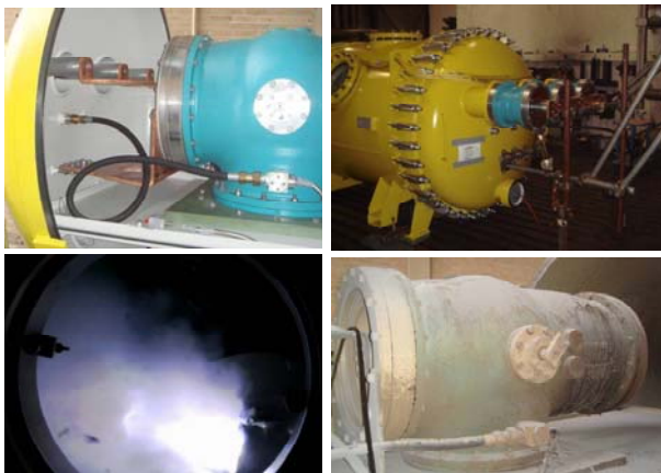
Figure 12: Arcing test of a 550 kV GIS component carried out in a testing vessel to absorb SF 6
