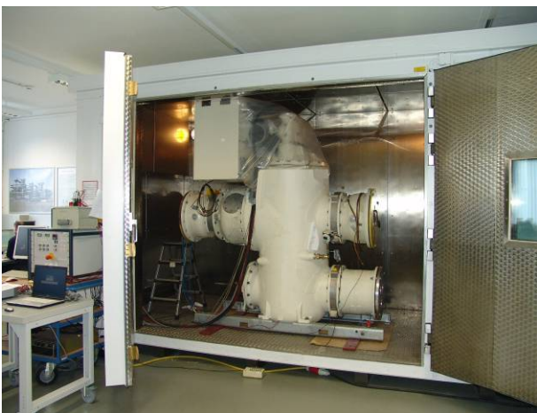
Figure 6: Example of a mechanical test at limit temperatures of a 145 kV GIS
