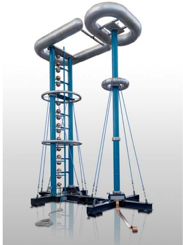
**Figure 2:** Picture of a Connection Point CO 1800 DOC (D => divider, O=> overshoot compensation C=> chopping gap).
