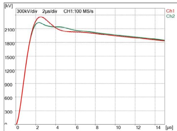
**Figure 5:** comparison between a compensated and uncompensated lightning impulse
