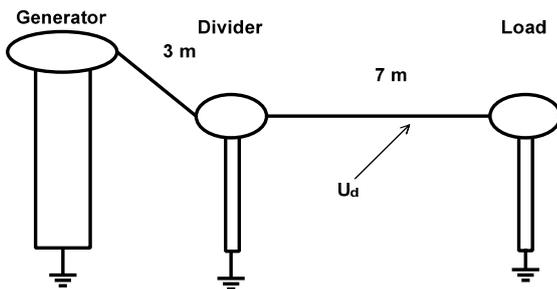
Figure 7: Test set-up 2
