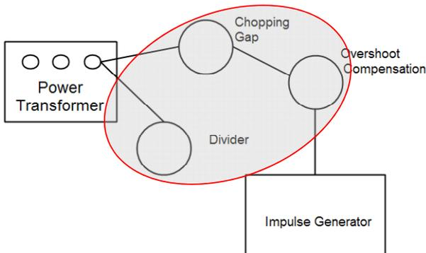
**Figure 1:** Common layout of an impulse test system containing divider, overshoot compensation and chopping gap.
