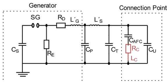
**Figure 4:** Equivalent circuit diagram of an impulse test system containing connection point.
