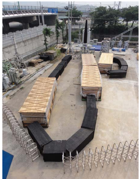
Fig. 2 Test Assembly – Assembled and After Filling with Sand and Fitment of Covers
