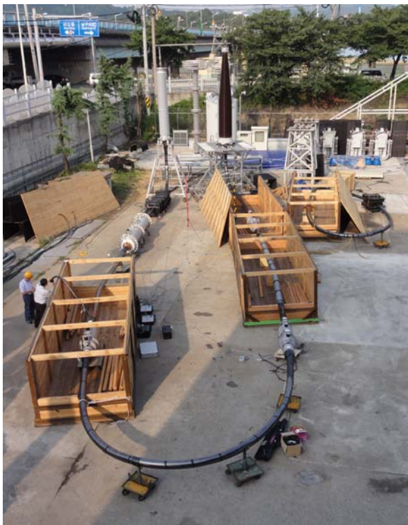
Fig. 2 Test Assembly – Assembled and After Filling with Sand and Fitment of Covers
