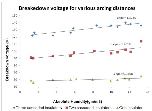
**Figure 6:** Growth in slope of breakdown voltage enhancement with the arcing distance increased by cascading similar insulators
