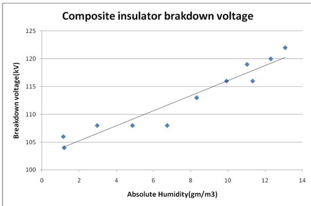
**Figure 4:** Breakdown voltage enhancement with absolute humidity for a composite insulator
