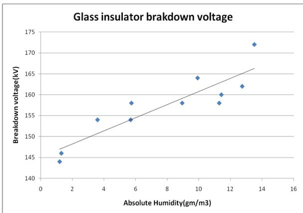
**Figure 5:** Breakdown voltage enhancement with absolute humidity for a glass insulator
