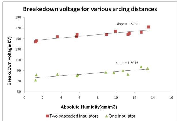
**Figure 7:** Growth in slope of breakdown voltage enhancement with the arcing distance increased by cascading another similar insulators
