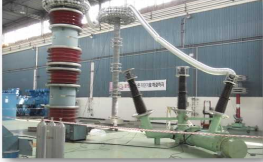
Figure 7: AC withstand voltage test equipment configuration
