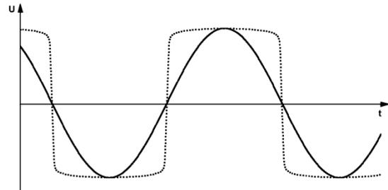
Fig. 3: Typical wave shape of a cosine-square wave (dotted) and sinusoidal VLF voltage
