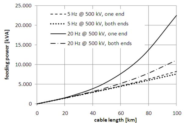
Fig. 6: Required feeding power at a test voltage of 500 kV depending on the cable connection
