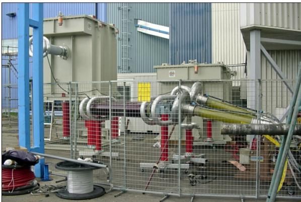
Fig. 2: Test of a HVDC submarine cable with two resonant reactors in series
