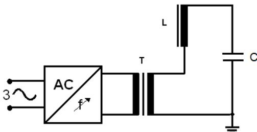
Fig. 1: Series resonant circuit with variable frequency
