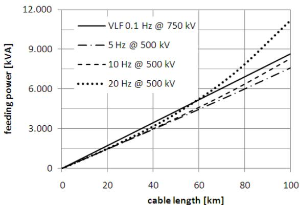
Fig. 5: Required feeding power at a test voltage of 500 kV (750 kV for 0.1 Hz), cable fed from both ends
