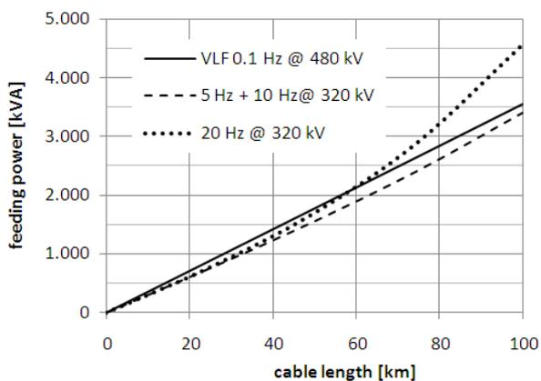
Fig. 4: Required feeding power at a test voltage of 320 kV (480 kV for 0.1 Hz), cable fed from both ends
