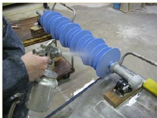
Figure 3: Example of pollution of the insulator in RRT test performed at NGK (adopted from [4]).
