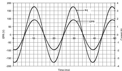
**Figure 2:** Injected AC current and tower base EPR ( $f=52\text{Hz}$ )
