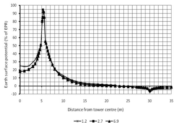
Figure 8: ESP profiles due to various rise times
