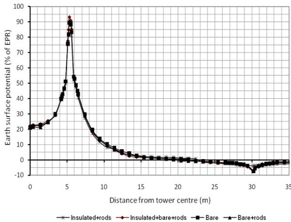
**Figure 11:** Influence of return electrode on ESP
