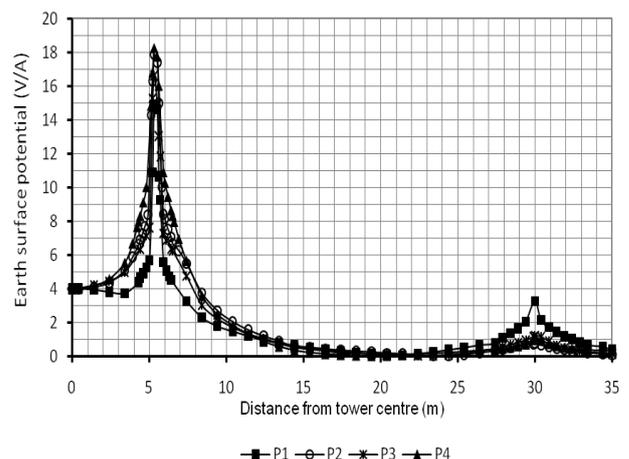
**Figure 10:** ESP profile over diagonal profiles under DC current
