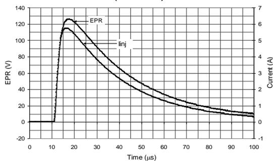
**Figure 3:** Impulse current and EPR
