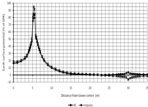
Figure 6: Comparison between ESP due to ac and impulse currents over profile P4
