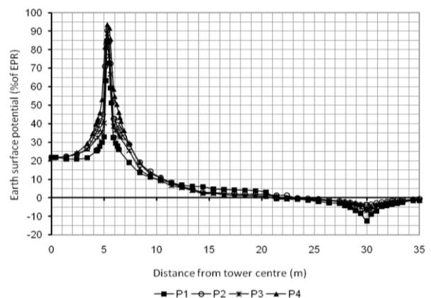
**Figure 11:** ESP profiles along each tower footing under impulse current
