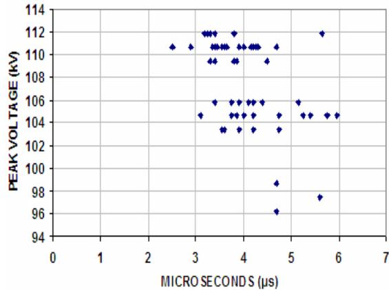
**Figure 9:** Peak Impulse Voltage (kV) against Time-to-Breakdown ( $\mu\text{s}$ ) for 125 mm Rod-Rod gap geometry.
