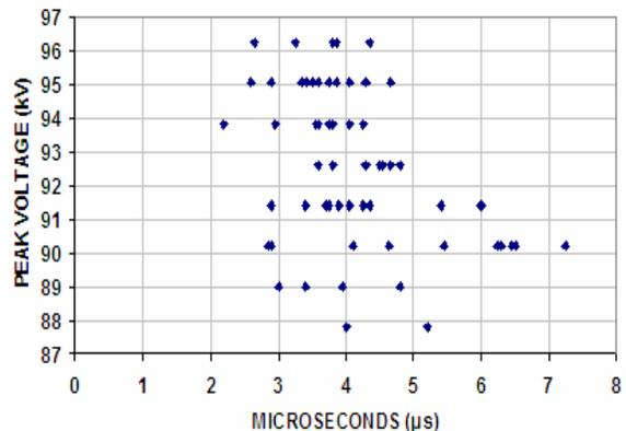
**Figure 10:** Peak Impulse Voltage (kV) against Time-to-Breakdown ( $\mu\text{s}$ ) for 100 mm Rod-Rod gap geometry.
