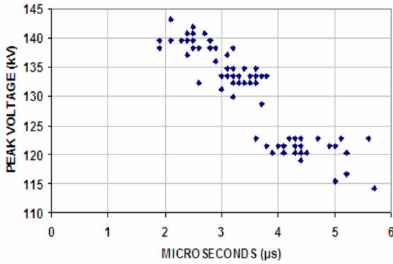
**Figure 8:** Peak Impulse Voltage (kV) against Time-to-Breakdown ( $\mu\text{s}$ ) for 150 mm Rod-Rod gap geometry.
