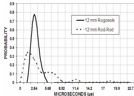
**Figure 2:** Distributions of time-to-breakdown for 12 mm gaps at mean probability of breakdown [5].
