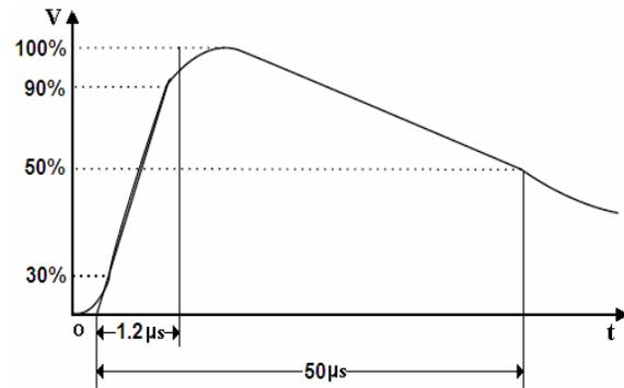
**Figure 4:** Illustration of a 1.2/50  $\mu$ s lightning impulse waveform as defined in the IEC60060-1: *High Voltage Test Techniques* [6].
