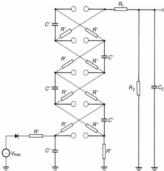
**Figure 3:** Multistage Marx Generator circuit used in the experiment. Adapted from Kuffel et al. [3].
