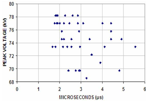
**Figure 11:** Peak Impulse Voltage (kV) against Time-to-Breakdown ( $\mu\text{s}$ ) for 75 mm Rod-Rod gap geometry.
