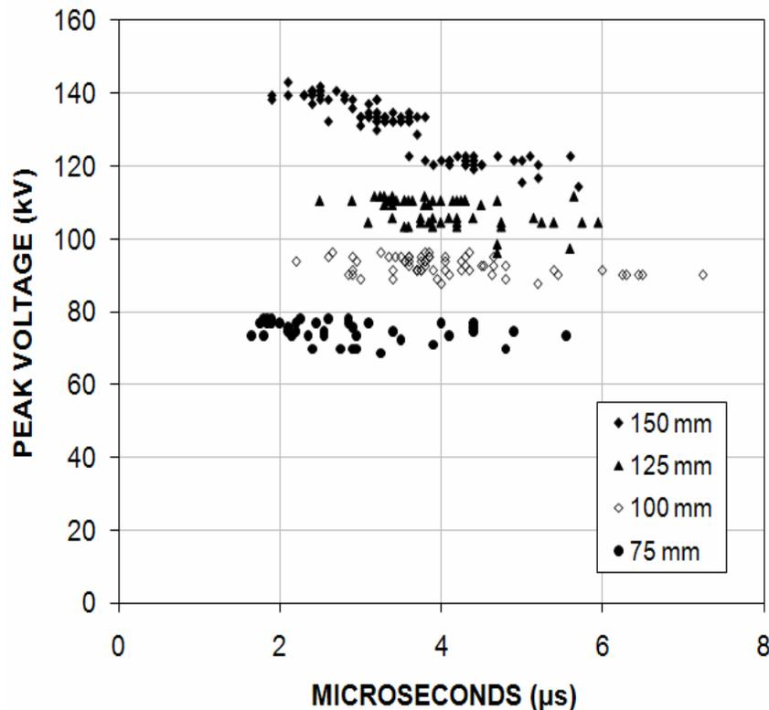
**Figure 7:** Peak Impulse Voltage (kV) against Time-to-Breakdown ( $\mu$ s) values for four gap sizes.
