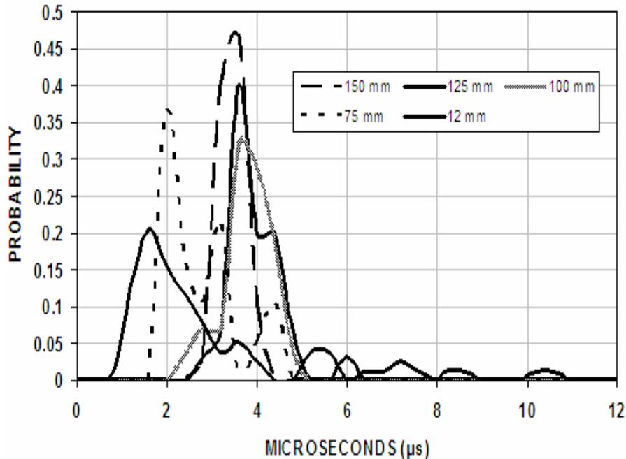
**Figure 12:** Distribution of time-to-breakdown results for all gap sizes including 12 mm gap results
