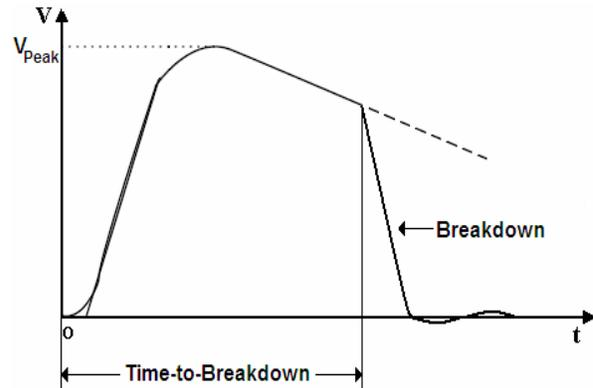
**Figure 5:** Illustration of voltage waveform when breakdown across the gap occurs.
