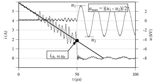
**Figure 2:** Current chopping with high frequency oscillation, 50 Hz component and transient recovery voltage
