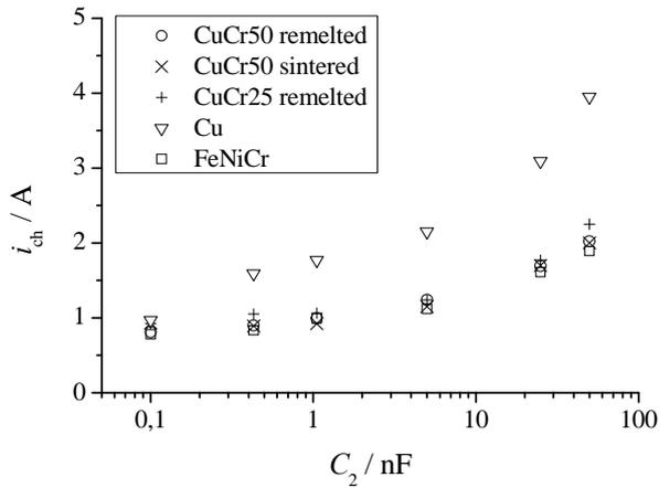
**Figure 3:** Dependence of parallel capacitance and chopping current for different materials with  $I = 630$  A
