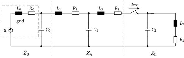
**Figure 1:** Applied test circuit
