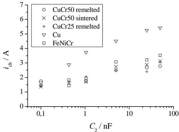
**Figure 4:** Dependence of parallel capacitance and chopping current for different materials with  $I = 150$  A
