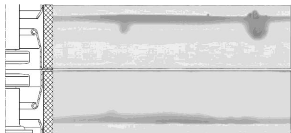
Figure 6: VI after 30 times of interrupting 5kA, polarity of current was changed after every switching operation
