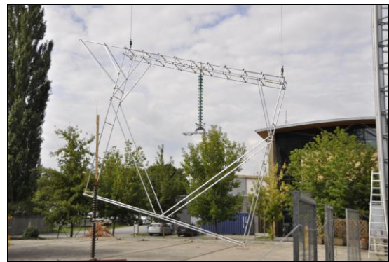
Figure 7. Full scale test model, here simulating displacement of insulator due to wind, an angle in the line or temperature - or ice load.
