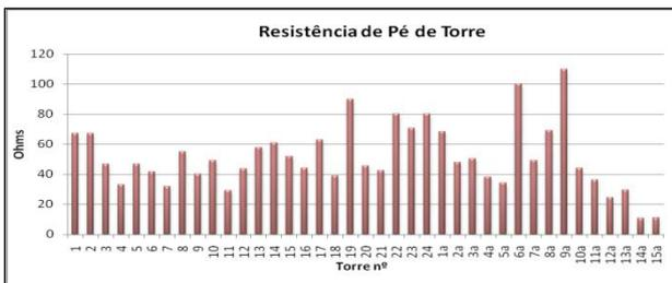
Fig. 4 – Ground Resistance Measurement
