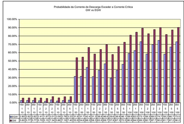
Figure 17 - Probability of Discharge Current Exceed the Critical Current
