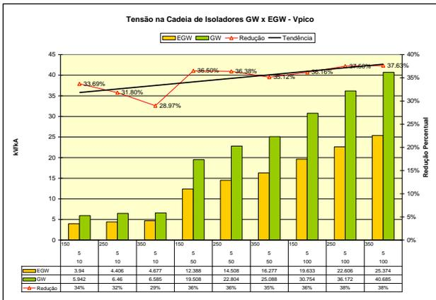
Figure 15 - Comparative Results - Time Front Wave Fixed in 5μs
