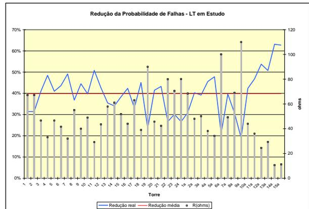
Figure 20 - Reducing the Probability of Failure as a Function of R (ohms) - LT Study
