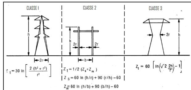
Fig. 2 – Approximations Surge Impedance  $Z_t$  for Geometry Classes [6]
