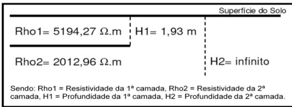
Figure 3 - Diagram of Soil Stratification in Two Layers
