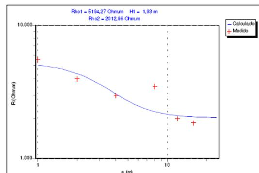
Figure. 2 – Soil Stratification Chart
