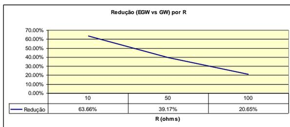
Figure 19 - Reduction EGW vs GW as a Function of Foot Tower Resistance
