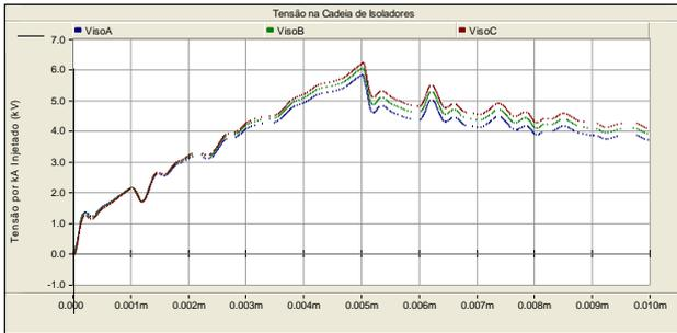
Figure 10 - Surge in insulation for Injection 1kA with 5µs front time wave
