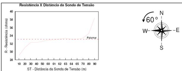
Fig. 5 – Result of Ground Impedance Measurement - Tower 4
