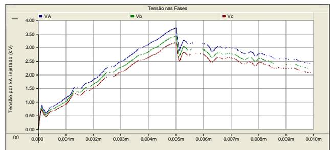
Figure 9 - Overvoltages phases for Injection 1kA with 5 $\mu$ s front time wave
