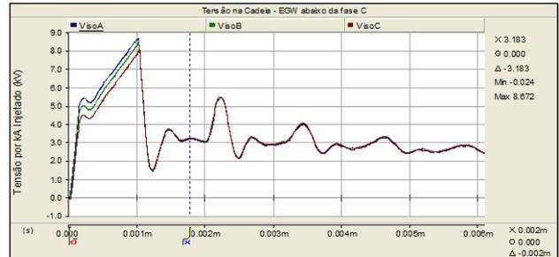
Figure 13 - Circuit-phase arrester cable with extra soil to 12.70 meters
