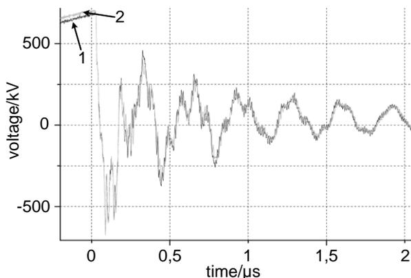
**Figure 5:** Comparison of VFTOs with a maximum amplitude of about 700 kV: The darker line represent VFTOs without rings (1). VFTOs with 6 ferrite rings are drawn in the brighter colour (2). No damping is visible.
