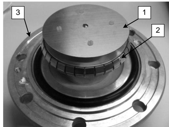
**Figure 3:** The capacitive sensor which was made at University of Stuttgart: It consists mainly of a double layer board (1) which forms a capacitive voltage divider. The board and a copper RF-seal (2) are mounted on a flange cap (3).
