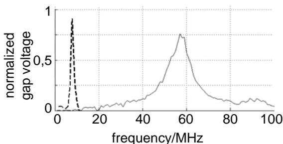
**Figure 8:** Gap voltage measured by a field probe as a function of frequency: Resonator without external capacitor parallel to the gap (grey curve) and Resonator with 5 nF capacitor parallel to the gap (dashed curve)
