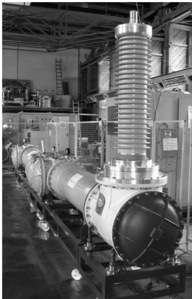
**Figure 2:** The high voltage test setup in the laboratory of University of Stuttgart: ABB 550 kV GIS type ELK-3 with bushing
