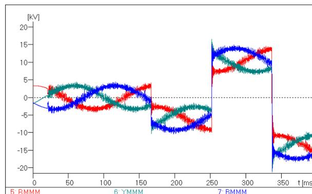
**Figure 7:** Motor terminal voltage-to-earth waveforms (including cycloconverter switching) with three consecutive arcing earth fault events on the red phase
