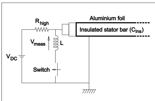
**Figure 3:** Laboratory circuit used to measure the high frequency losses of motor stator bar insulation
