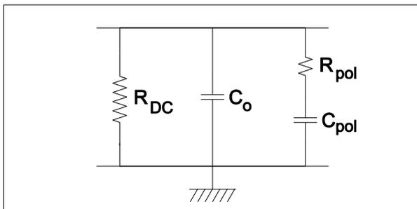
**Figure 2:** Assumed model of the epoxy-mica motor insulation-to-earth
