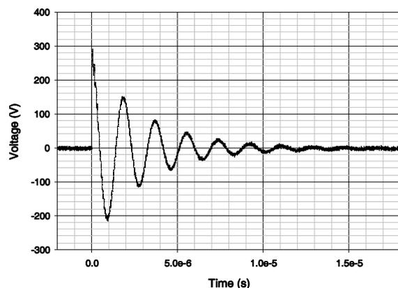
**Figure 6:** Discharge voltage waveform when the stator bar capacitance-to-earth was discharged through the same inductor
