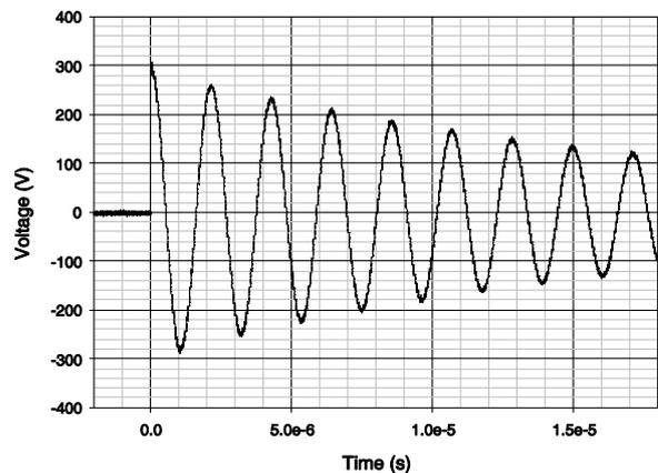
**Figure 5:** Discharge voltage waveform when a low-loss capacitor was discharged through the inductor
