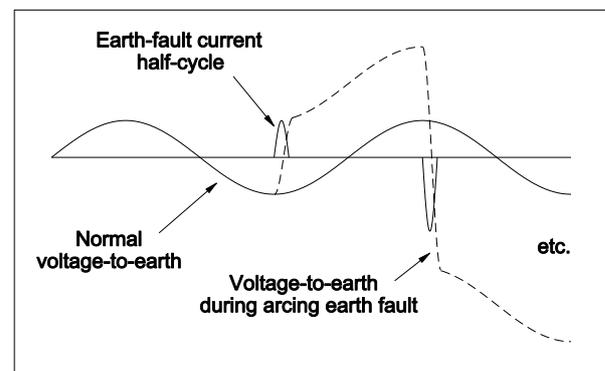
Figure 1: Waveforms for an arcing earth fault [1]
