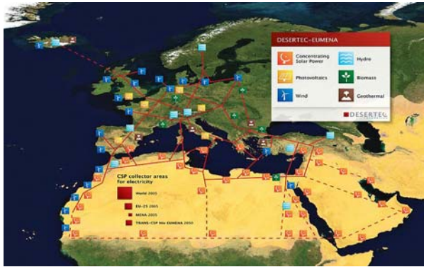
Figure 2: The Desertec plan. Europe will be interconnected with HVDC links in order to exploit the energy of the sun in the south and the wind rich in the north in order to supply a steady energy to customers around the continent [5].
