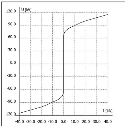
Fig. 3. Characteristic Curve: Medium Voltage MOV
