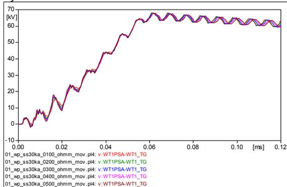
Fig. 5. Overvoltages induced on the MV side with variation of the soil resistivity: WT1
