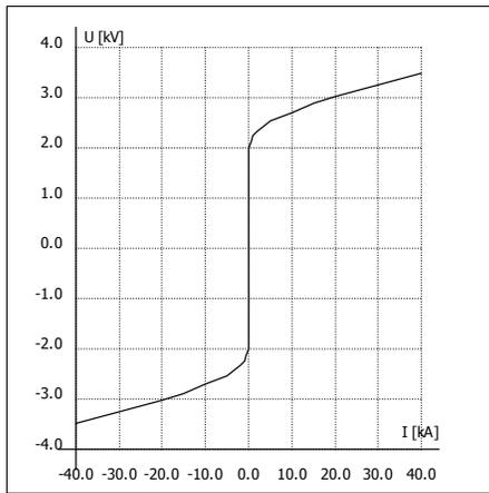
Fig. 2. Characteristic Curve: Low Voltage MOV
