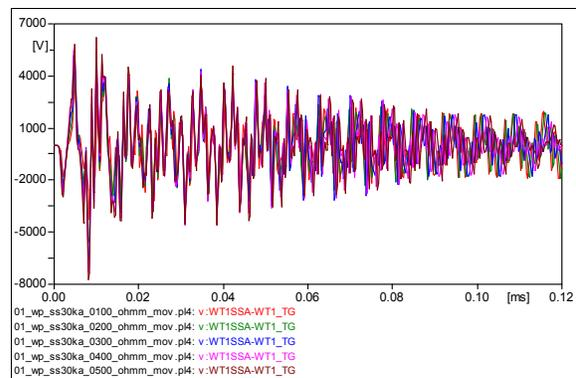
Fig. 4. Overvoltages induced on the LV side with variation of the soil resistivity: WT1
