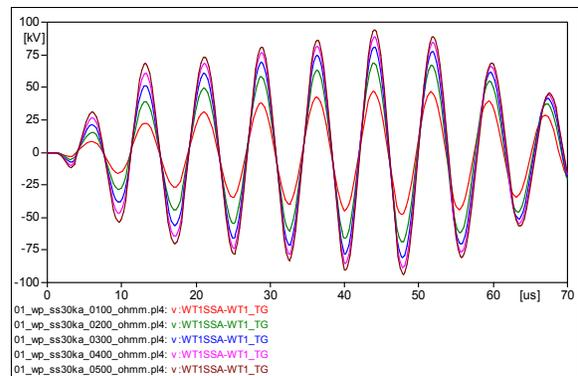
Fig. 1. Overvoltages induced on the LV side with variation of the soil resistivity: WT1
