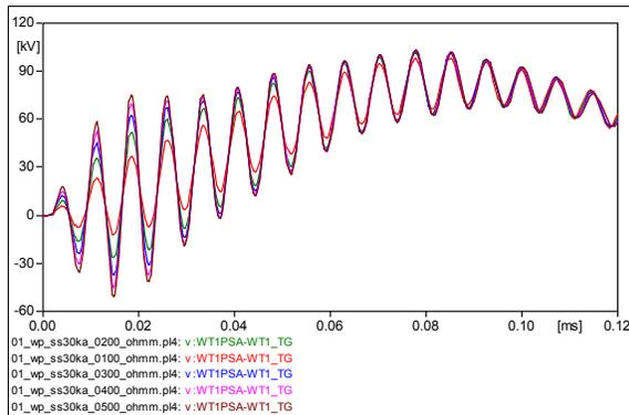
Fig. 2. Overvoltages induced on the MV side with variation of the soil resistivity: WT1
