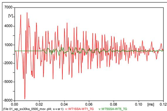
Fig. 6. Delay in the induced overvoltages (LV side) caused by travelling waves between the WT1 and WT5 with the MOVs connected (Soil resistivity 500  $\Omega\text{m}$ )
