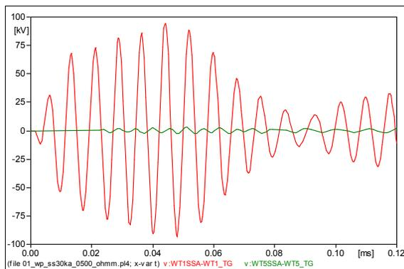
Fig. 3. Delay in the induced overvoltages (LV side) caused by travelling waves between the WT1 and WT5 (Soil resistivity 500  $\Omega m$ )
