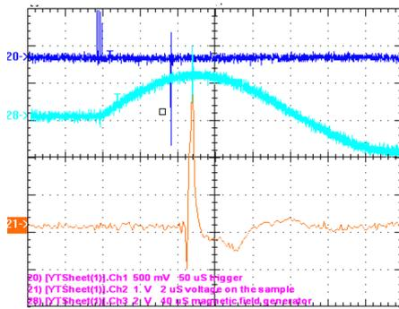
**Figure 9:** The typical waveforms of flashover
