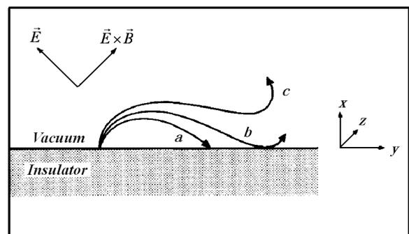
**Figure 1:** Electron trajectories in SEEA for three different magnetic fields and for emission normal to the surface
