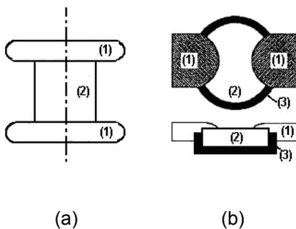
**Figure 3:** The structure of the electrode: plane-shaped (a) and finger-shaped (b). Electrode is labeled as (1), dielectric is labeled as (2) and Teflon holder is labeled as (3)
