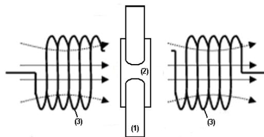
**Figure 5:** The arrangement of electric field and magnetic field. Electrode is labeled as (1), dielectric is labeled as (2) and solenoids is labeled as (3)
