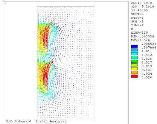
Figure 8: The vector diagram of the magnetic flux
