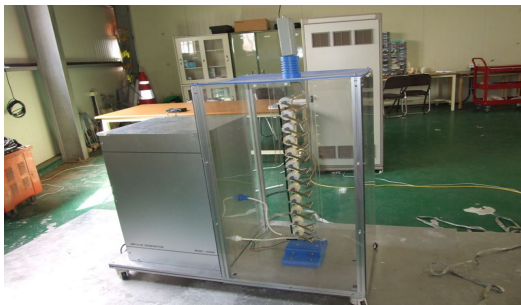
Figure 5: Impulse generator used for the down scaled simulation test
