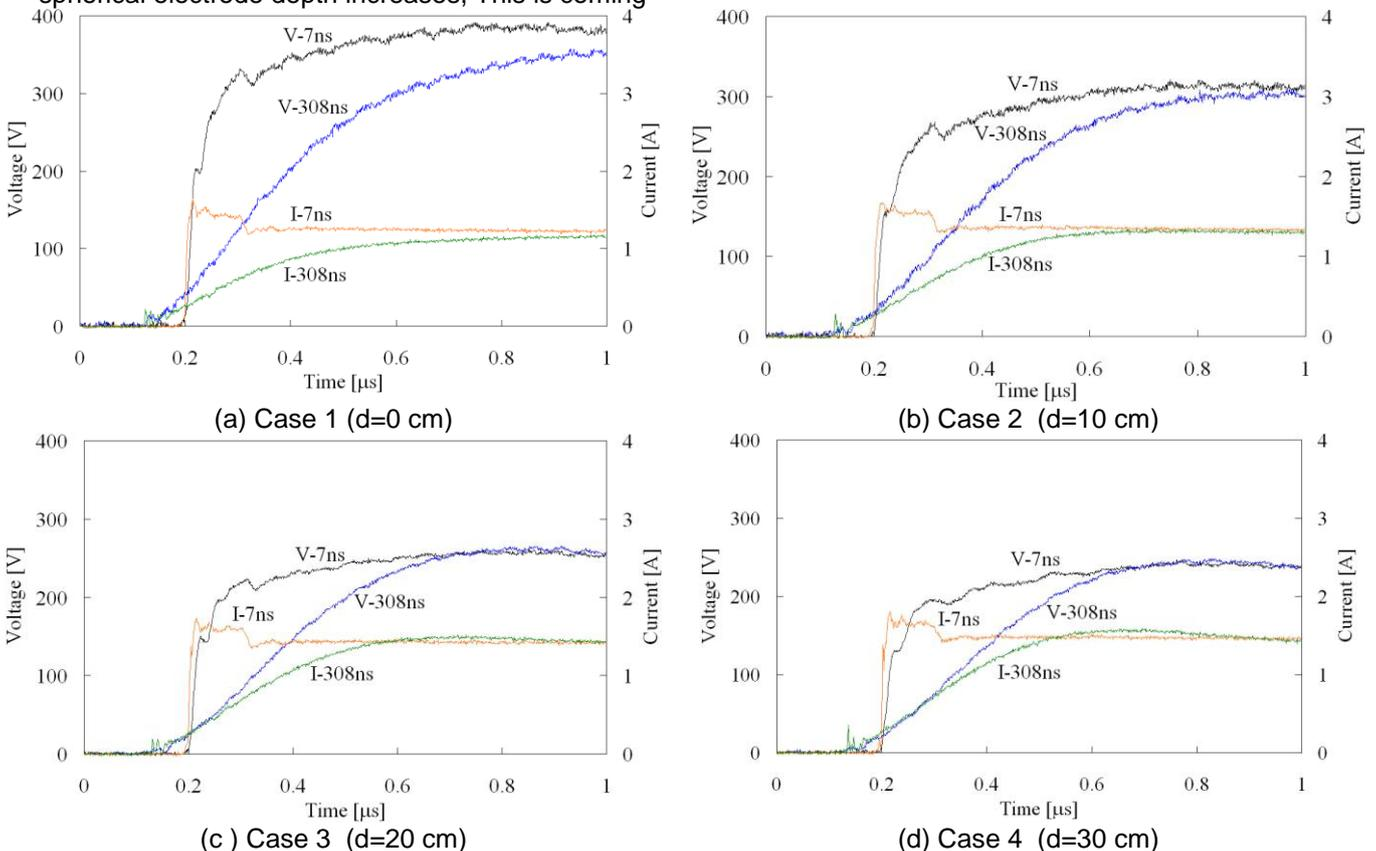
**Figure 3:** Measured voltages and injected currents of rise times 7 and 308 nsec
