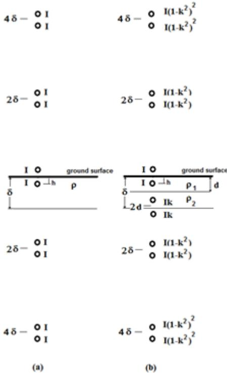
**Figure 6:** Image maps for a) homogenous soil and b) two-layer soil
