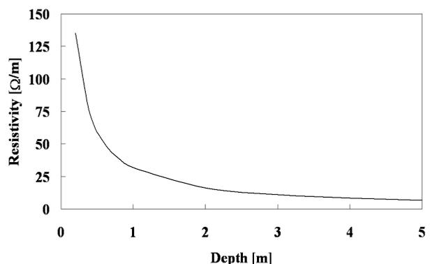
Figure 2: Soil resistivity vs. soil depth
