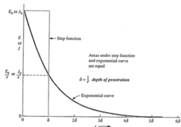
**Figure 5:** Electric field  $E$  or current density  $J(=\sigma E)$  as a function of depth of penetration [16]
