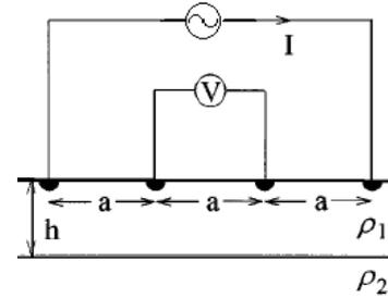
Fig. 1. Wenner's four-probe test system for a three-layer earth model.
