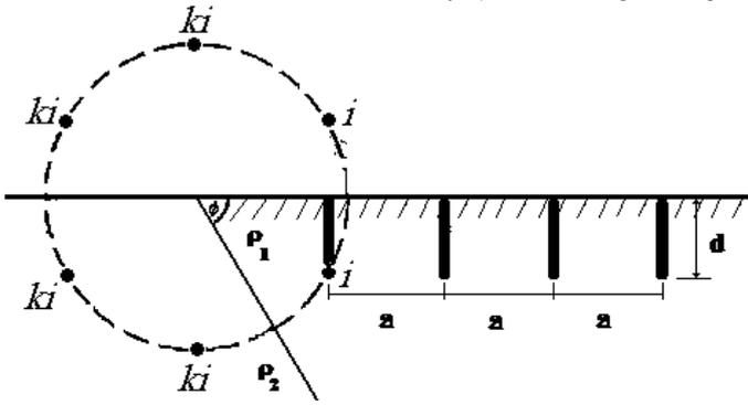
Fig. 2. Images of spherical elements for four electrodes in sloped top layer
