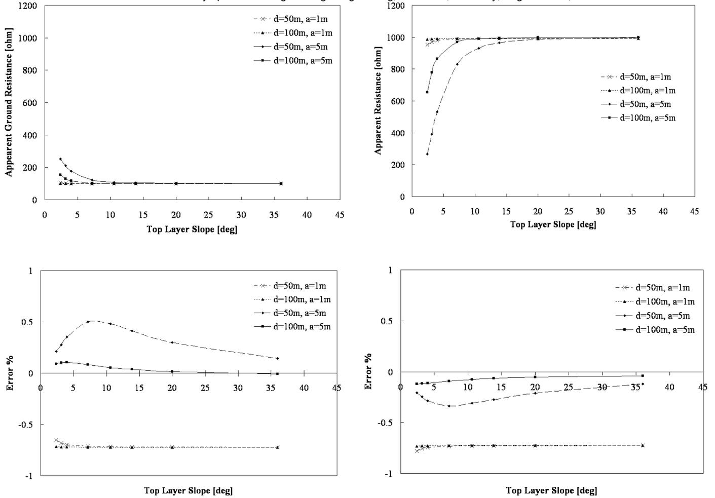
Fig. 4 Case 1– Error % of apparent resistivity vs. top layer slope
