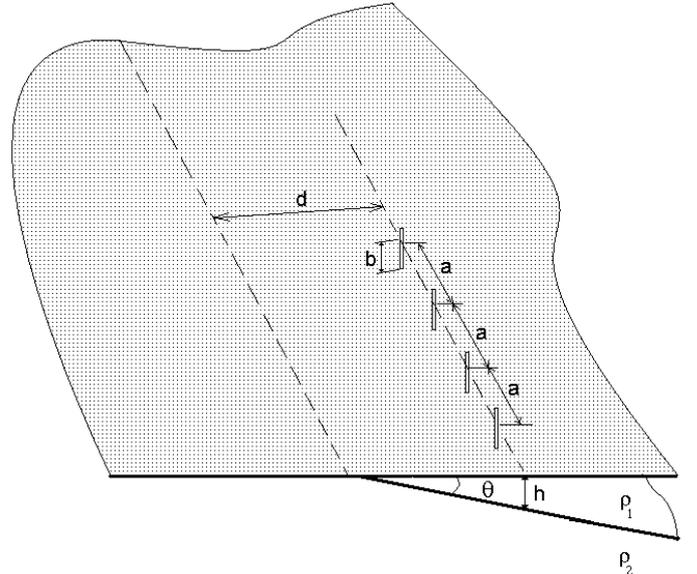
Fig. Measurement of the ground resistivity by using four probe method in sloped top layer ground
