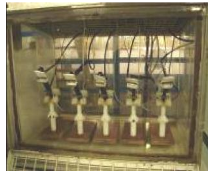
Figure 5: Test equipment for tracking test
