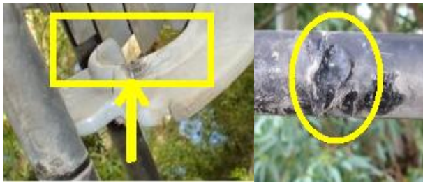
Figure 3: Sample of electrical tracking and erosion
