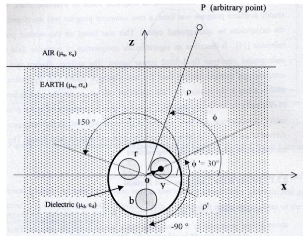
**Figure 3** Cross section of an under ground cable and various angles physical parameters
