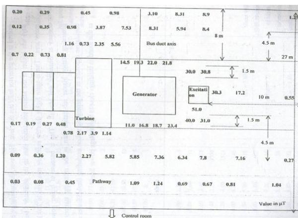
**Figure 5** Layout of area around 210 MW generator and results of spot measurement
