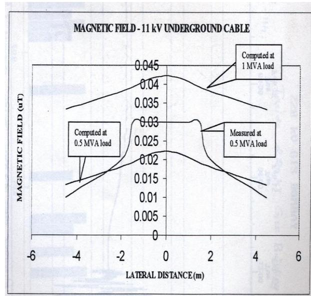
**Figure 4** Lateral Magnetic fields of 11kV under ground cables
