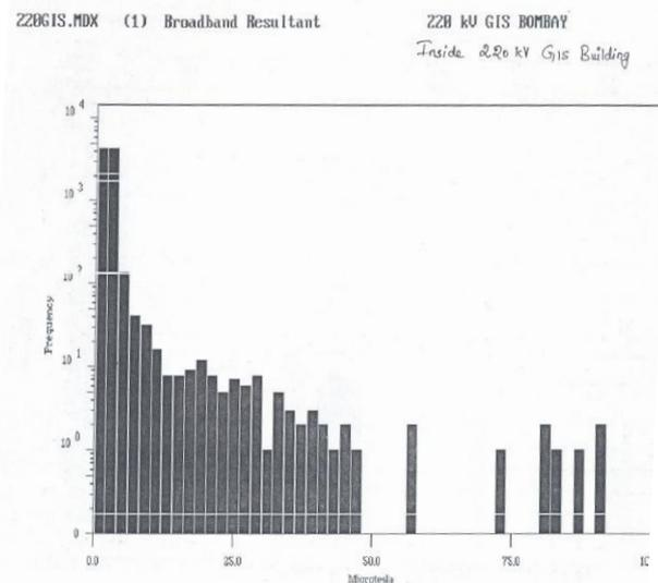
Figure 3: Histogram of magnetic fields measurement in 220 kV GIS building
