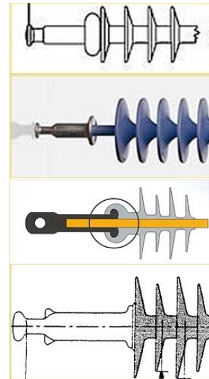
Figure 6: Examples of four typical end fitting designs.
