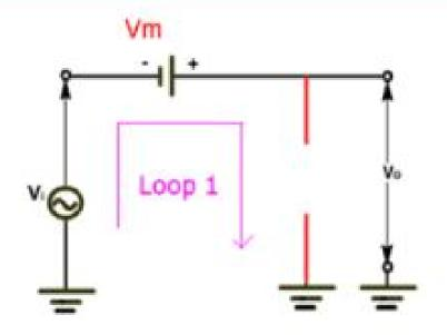
During the + ve cycle diode turns off
