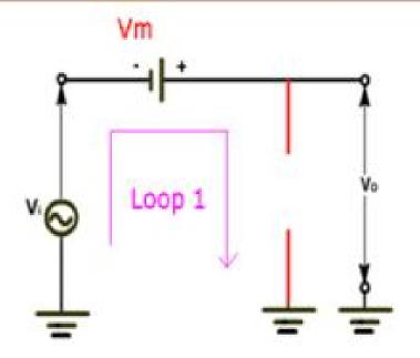
During the + ve cycle diode turns off
