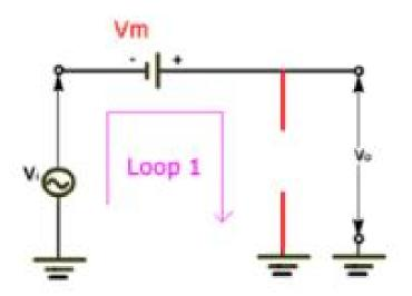
During the + ve cycle diode turns off
