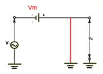
During the -ve cycle diode turns on
